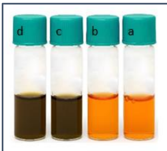
Figure 2: The prepared samples of a) pure P3HT, b) 0.1, c) 0.3, and d) 0.4 wt% Ag NPs.
